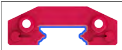
Standard wiper (blue contour = contact surface)
