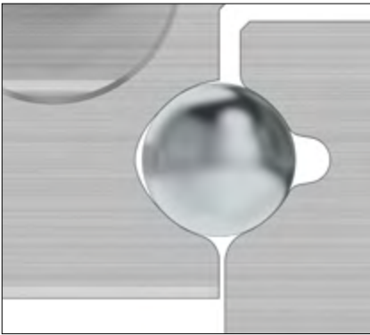
Gothic arc profile of the guideway tracks
