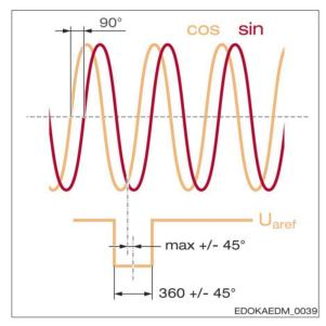
$\boldsymbol{U}_{\text{aref}}$  Starting voltage of the reference signal
