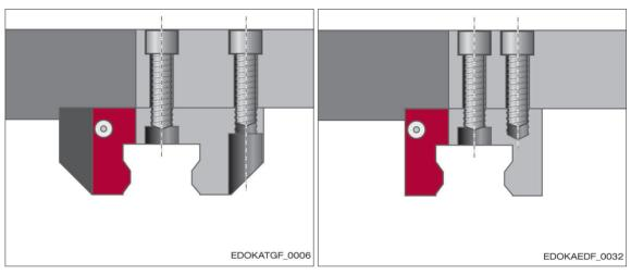
Attaching using the tapped hole
