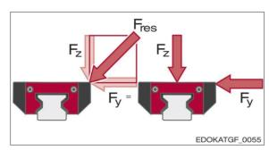
Vector addition of the horizontal  ${\bf F_{\rm Y}}$  and vertical  ${\bf F_{\rm Z}}$  force components for the total load  ${\bf F_{\rm res}}.$
