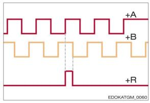
Signal waveform of the digital interface
