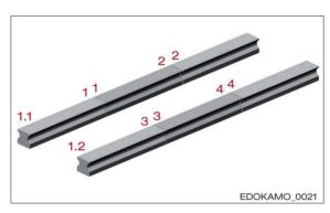
Numbering of the guide rail joints and set numbers The notation 1.1 only refers to the GP design.
