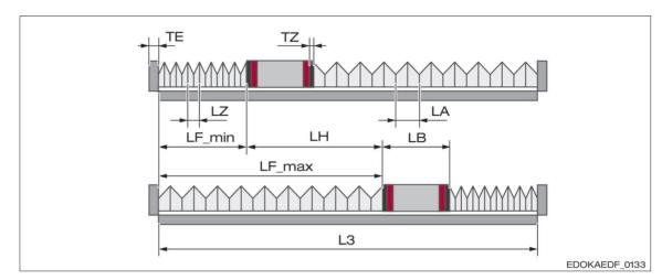
Lengths of one guide rail with one carriage:
