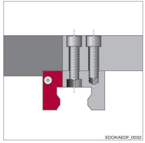
Carriages with blind fxing holes fastened from below
