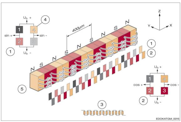
Schematic sensor structure:
