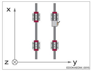
Reading head arrangement for a vertical axis
