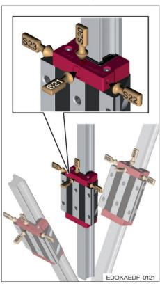
Oil lubrication for vertical installation and installation inclined around the transverse axis
