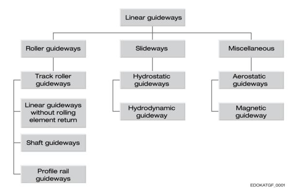
Roller guideways can also be subdivided according to the type of rolling element movement within the guideways into roller guideways with and without a rolling element recirculating unit. In the case of guideways without a rolling element recirculating unit, the stroke is limited by the length of the guiding components. Guideways with a rolling element recirculating unit, which include the SCHNEEBERGER profile rail guideways, have a theoretically unlimited stroke, which is
