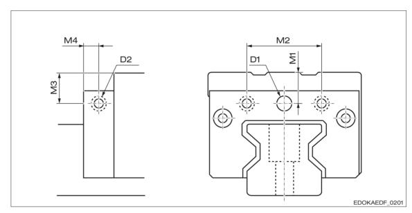
Connecting thread in the front plate front and side:
