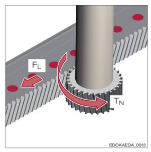
Rack with longitudinal force  $\mathbf{F}_{_{\mathrm{I}}}$  and pinion with torque  $\mathbf{T}_{_{\mathrm{K}}}$
