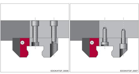
Carriages with continuous tapped fixing holes fastened from above
