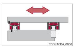
Both guide rails and a carriage side with a datum edge, a guide rail and its carriages also with side fastening
