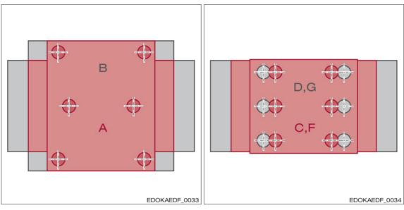
Screw drilling templates for carriage type A and B
