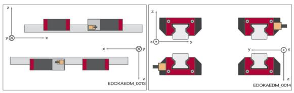
Reading head arrangement for a horizontal axis
