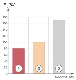
Push force based on the example of a ball guideway BM 35. The push force  $F_{\nu}$  (%) of wiper variants is illustrated in relation to a standard wiper (100%).
