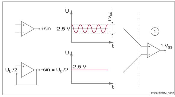
Signal reading head for analogue systems, operational amplifier output, differential output with fixed reference voltage
