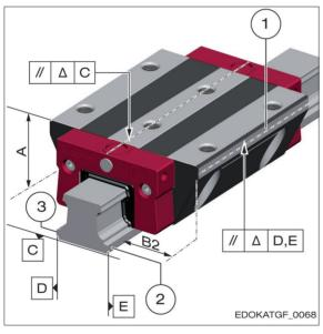
Tolerances of reference measurements for carriages to the guide rail
