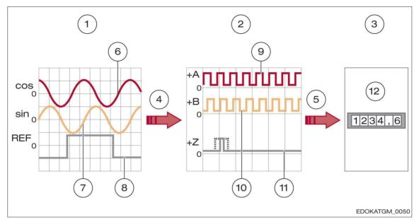
The analogue input signals (sin, cos, Ref) are interpolated (red arrow) with the digital output signals (+A, +B, +Z). Inverted signals are not represented:
