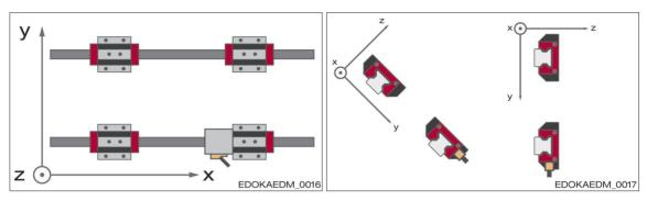
Reading head arrangement for the horizontal axis with wall assembly; rotated 90° around the longitudinal axis or inclined installation, e.g. inclined 45° around the longitudinal axis
