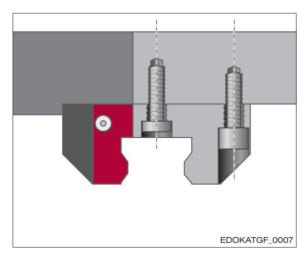
Attaching using the tapped hole
