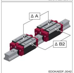
Maximum dimensional difference between the carriages on a guide rail:  $-\Delta A/\Delta B2$
