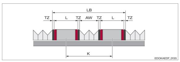
Lengths of one guide rail with two carriages and bellows:
