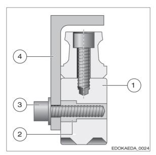
Transport fixture for guide rail with rack
