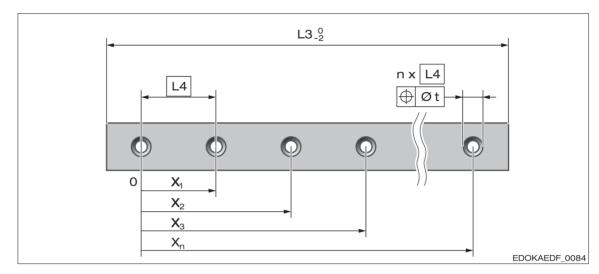
Diagram of fixing hole spacing L4:
