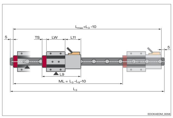
Maximum usable length ( $L_{max} = L3 - 10$ ) and measuring length (ML = L3 - L9 - 10):
