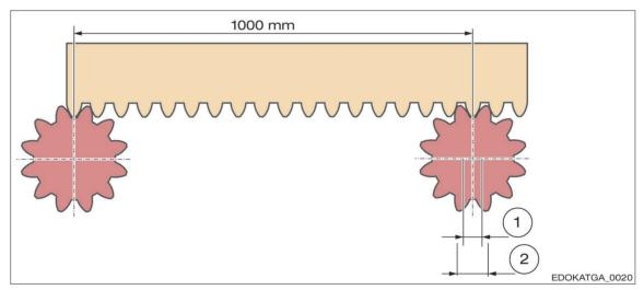
Example for 1000 mm travel distance for tolerance Q5 and Q6.
