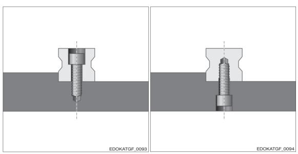
Guide rail with continuous fixing hole
