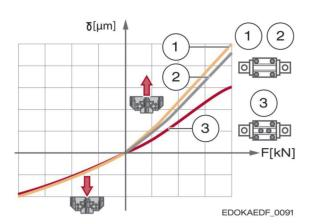
Influence of carriage fastening on rigidity based on the example of a 4-row ball guideway with 0-geometry. The force F (kN) under tension and pressure is applied against the deformation  $\delta$  ( $\mu$ m).
