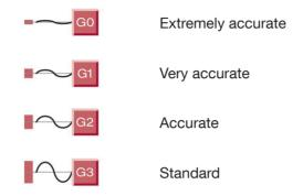
The accuracy classes determine both the tolerances of the reference sizes of the carriages to the guide rail, see the following image and Section 4.6.2 - Accuracy - Dimensional tolerances, and running accuracy of carriages on guide rails in accordance with Section 1.6.3 - Accuracy - running accuracy.
