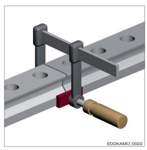
Installation using a fixing bridge
