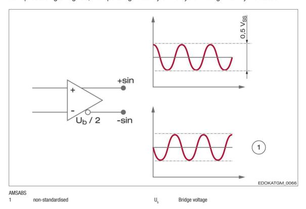
Signal waveform of the synchronous-serial interface with analogue signal, connection between the SSI values and the analogue signals:
