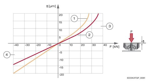
Deformation  $\delta$  (µm) is applied against the load F (kN) and results in compressive rigidity or tensile rigidity.
