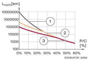
Nominal service life as a function of preload and force based on the example of an MR 45 roller guideway. Ratio P/C (%) with equivalent force P (N) and dynamic load capacity C (N) is applied against the nominal service life  $L_{\rm mm}$  (km).
