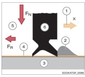
The function of a cross wiper (cross-section) in the direction of movement (yellow arrow).
