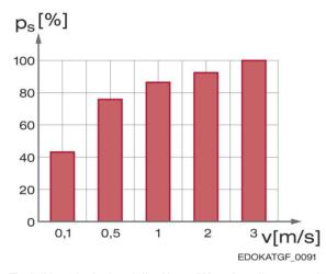
The build-up of noise by a ball guideway BM 25 depending on speed. Speed v (m/s) is plotted against sound pressure  $p_{\rm S}$  (%). Lubrication is provide by means of oil.
