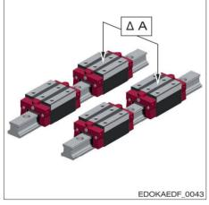
Maximum dimensions difference in carriages for two or more parallel guide rails, standard:
