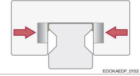
Contact surface area between tracks. Not suitable for guide rails with AMS!
