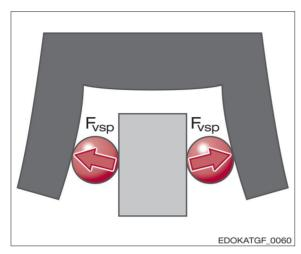
Preload force  $\mathbf{F}_{\mathbf{vso}}$  generated by rolling elements, which acts against the carriage. The figure shows a finished ground carriage top.
