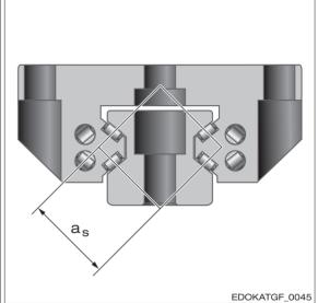
X-geometry with spacing a
