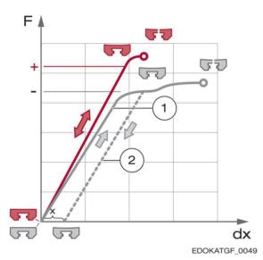
Force F is applied against deformation dx up to breaking point. In case of excessive loading an inductively hardened carriage is subject to plastic deformation; deformation x continues to occur.
